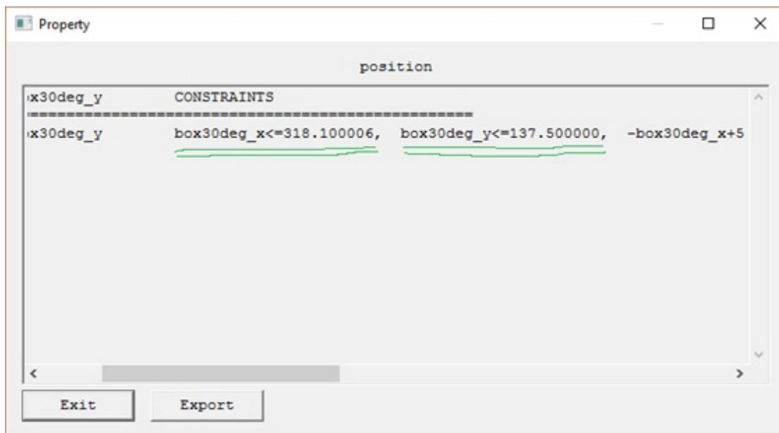
FIGURE 2.6: The query result that requests the position of the top-right corner of projectile launched at 30^\circ , at time t = 3.5s . The underlined parts of the result belong to the top-right corner point.
